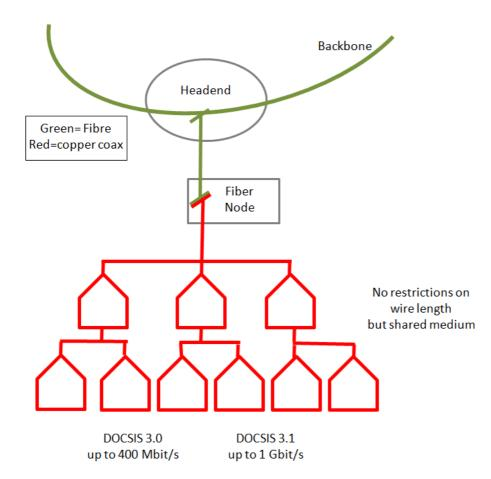
Figure 4: Broadband architecture based on the cable-TV network
