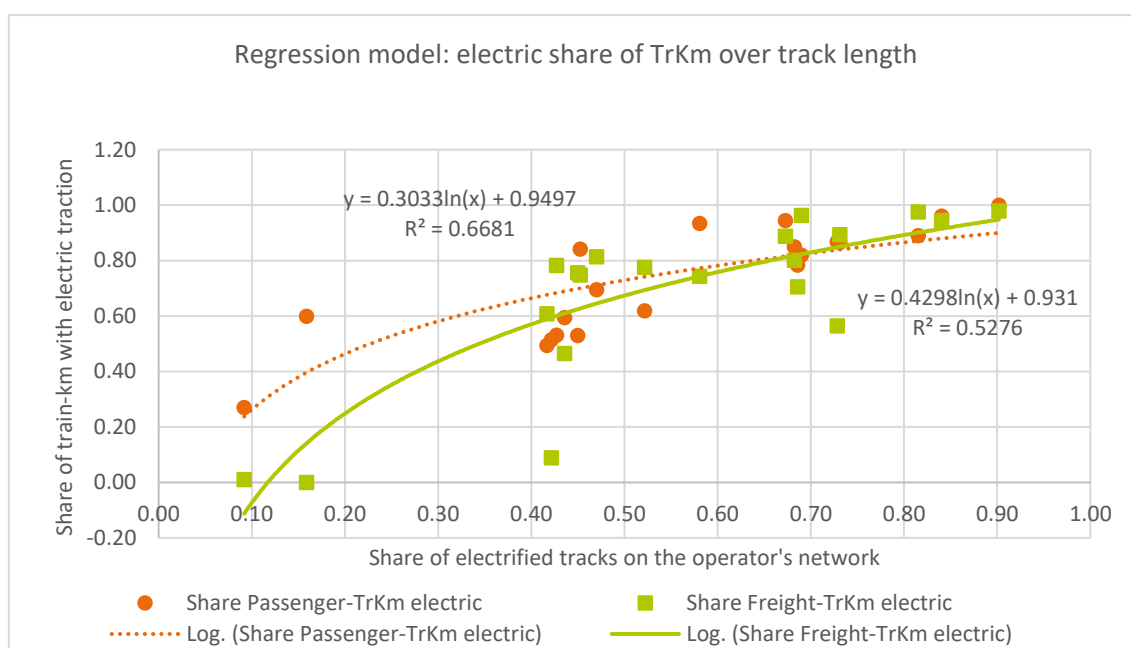
Figure 4.1: Model estimation for pkm and tkm by traction type over network electrification
