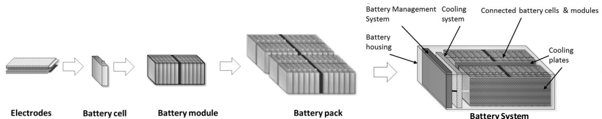
Figure 1: Schematic overview of the key components of a battery system after (Hettesheimer 2017)
