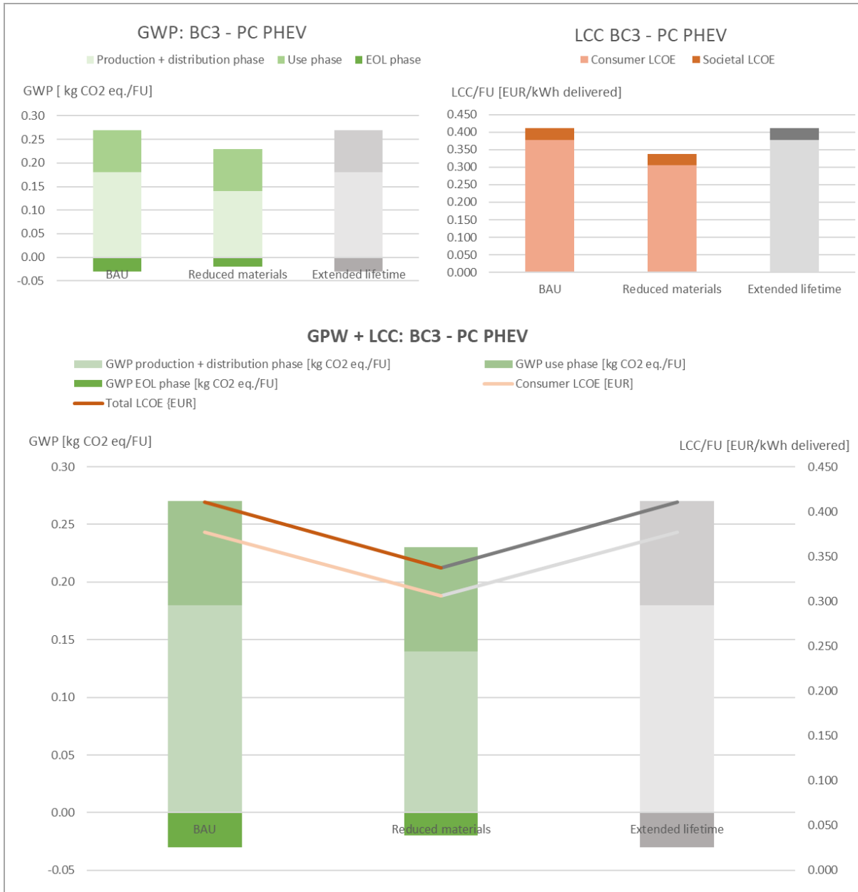
Figure 5: Ranking of the design options for BC3 – passenger car PHEV 18 .
