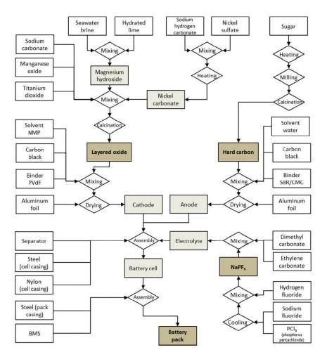
Figure 1: Cradle to gate diagram of sodium-ion production processes (Source: Peters et al (2016)<sup>5</sup>)
