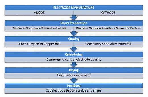
Figure 31: General process of electrode manufacturing for batteries<sup>125</sup>.
