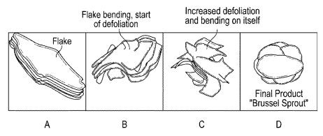
Figure 44: illustration of flake re-shaping transformation process. A: pure graphite flake, B: After substantial impacts with the processing equipment, the flake starts to bend and partially disintegrate at the edges, C: After further processing more substantial defoliation and dislocation of the flake occurs and more substantial bending of these defoliated layers, D: final product, the approximately spherical, rounded particle<sup>192</sup>.
